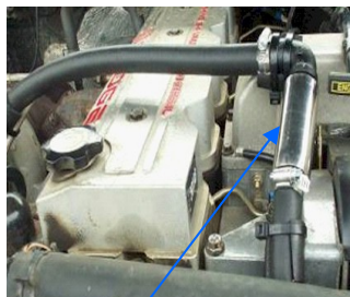
5.9 Cummins Engine Installation. Note the minimum 45 degree angle from vertical.
